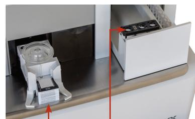
Load TT<sub>4</sub> slide here      Load reagent here
