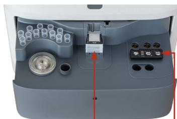
Load TT<sub>4</sub> slide here      Load reagent here
